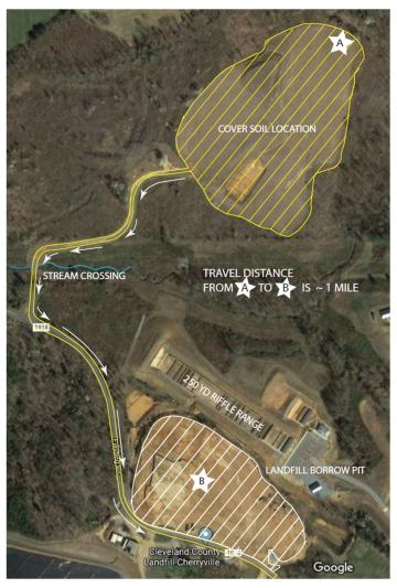
The volume of cover soil will be verified by survey. There could also be a measurement using a drone LIDAR for the borrow pit
